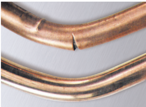
Figure 76. Copper bonded and copper clad earth rods.
